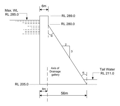
*The figure above shows the section of concrete gravity dam (non-overflow portion)*
